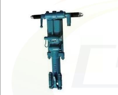
Hand held Rock Drill Model Y26 is mainly used for drilling, second blasting and other works in mines, railway, and water conservancy projects. It is designed for both dry and wet rock drilling on hard and medium hard rocks, and drilling vertical down or declined blast hole.
