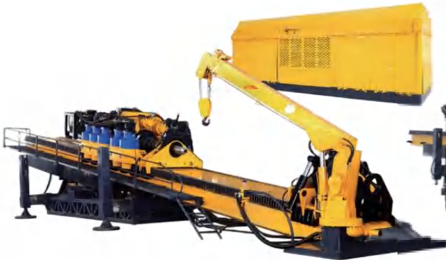
Model FDP-1000 Max. Pullback Force: 1000 t
