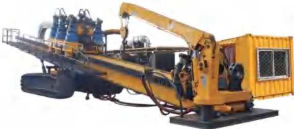
Model FDP-550 Max. Pullback Force: 550 t
