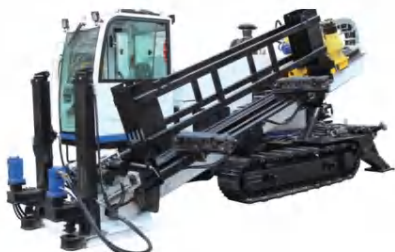
Model FDP-25 Max. Pullback Force: 25 t
