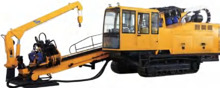
Model FDP-200/300 Max. Pullback Force: 200/300 t
