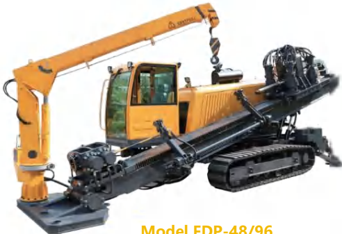
Model FDP-48/96 Max. Pullback Force: 48/96 t
