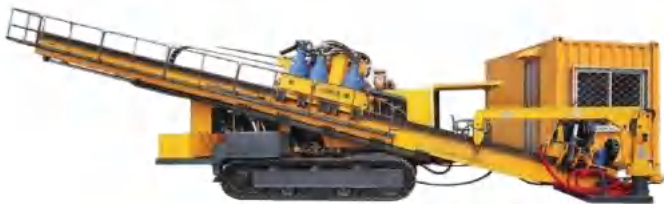
Model FDP-400 Max. Pullback Force: 400 t
